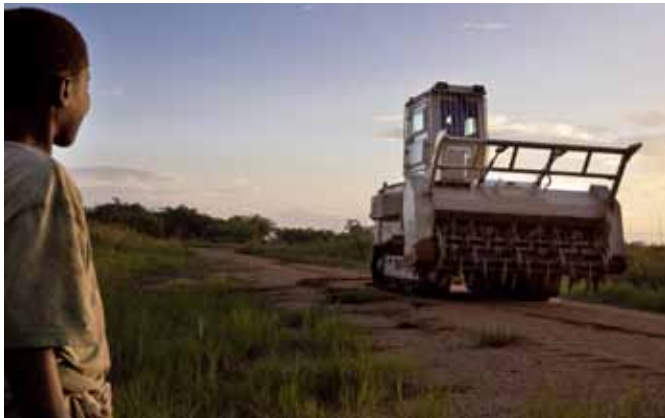
MineWolf 330 mine clearance machine returning to base after operations near Kisangani, DRC
